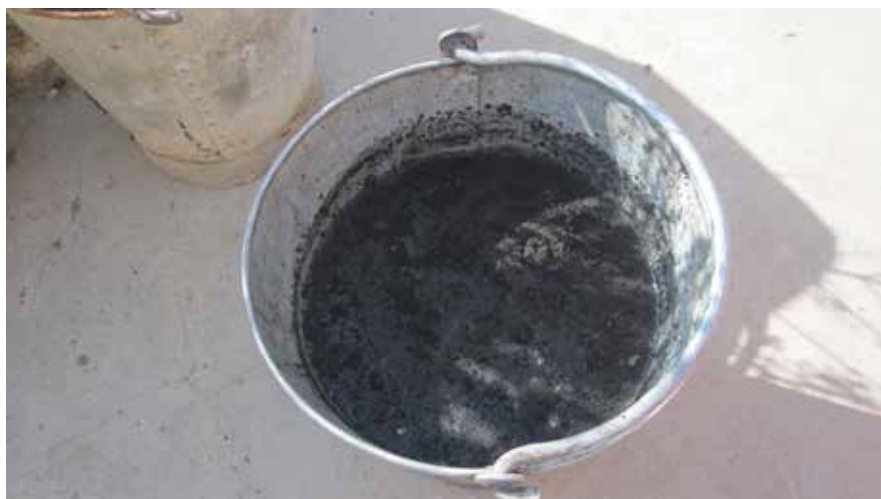
Tar collected from the smokeless chulha which can later be used for plants as a fertilizer
